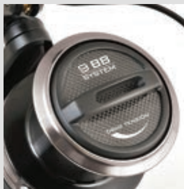
The advanced drag system is based on large diameter's disks, in order to disperse heat. The drag box is sealed by a rubber lining which keeps water and dust away.
