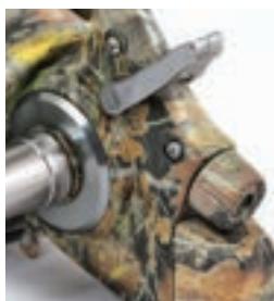
The special frame which follows the spool during its oscillation has two arms which avoid line to slip below the spool's skirt, thus avoiding dangerous tangles.
