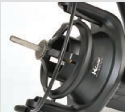
The special frame which follows the spool during its vertical oscillation has two arms which prevents line from slipping below the spool's skirt, thus avoiding dangerous tangles.
